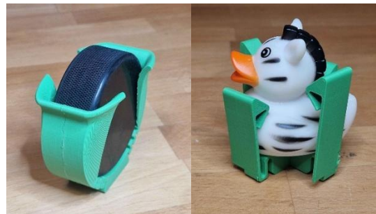
Figure 7: Manufactured payload mechanisms: cargo clamp and passenger restraint [1].
